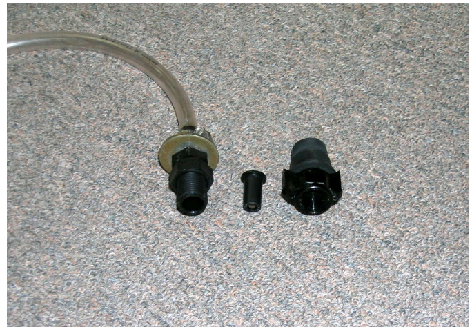
Figure 4- Check valve partly disassembled.
