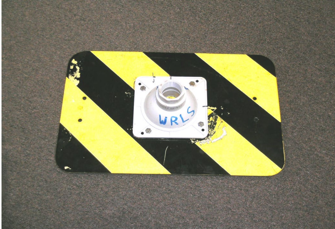
Figure 1- Example of base plate with drain.
