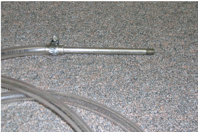
Figure 5- Valve stem to connect to air pump.
