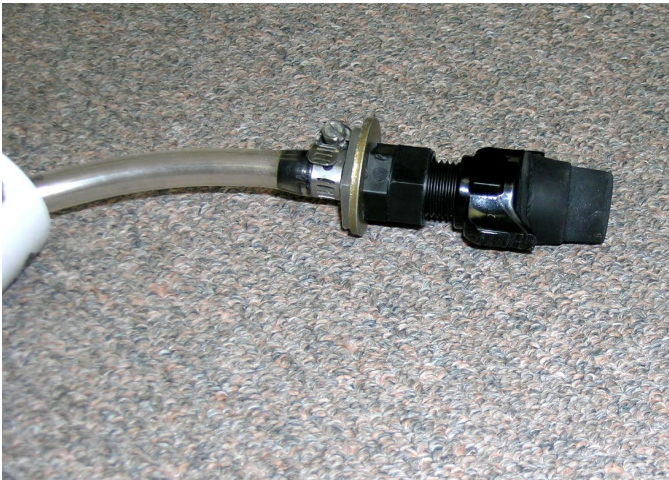
Figure 3- Check Valve Assembly with plug.
